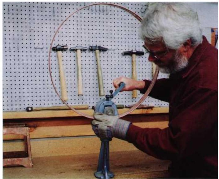
Figure 14. The author using the rim-rolling machine to make the second roll.
