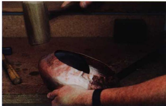
Figure 3. Regulating the bottom bowl section of the lamp using a wooden mallet over a steel "mushroom" stake.
