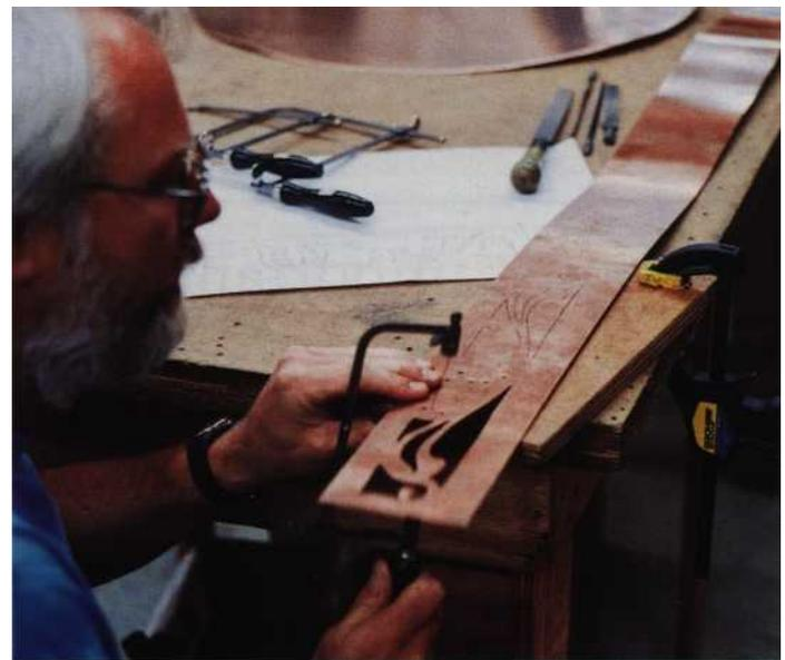
Figure 21. The time-consuming task of cutting out the intricate pattern in the "flat-top" shade. This particular band is 75" long and is going on a 24" diameter chandelier.
