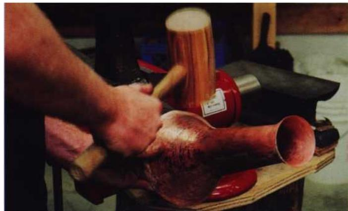
Figure 4. The "trumpet" section further along in the shaping process being regulated with a mallet over a curved stake.
