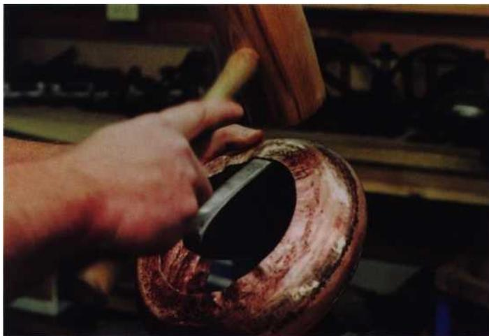
*Figure 6. The bottom bowl section has been partially planished and it continues to need regulation with the mallet.*
