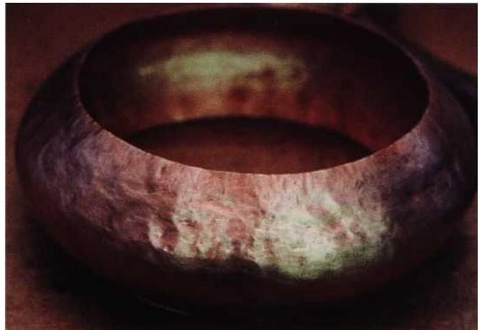
Figure 19. The bottom bowl section of a "rivet base" table lamp before planishing. Notice the ugly working hammer marks that contrast dramatically with the next photo of a "warty" style table lamp.
