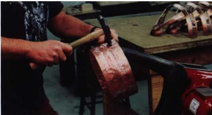
Figure 1. The beginning phase of "raising" the bottom bowl section of a "rivet-base" table lamp.
