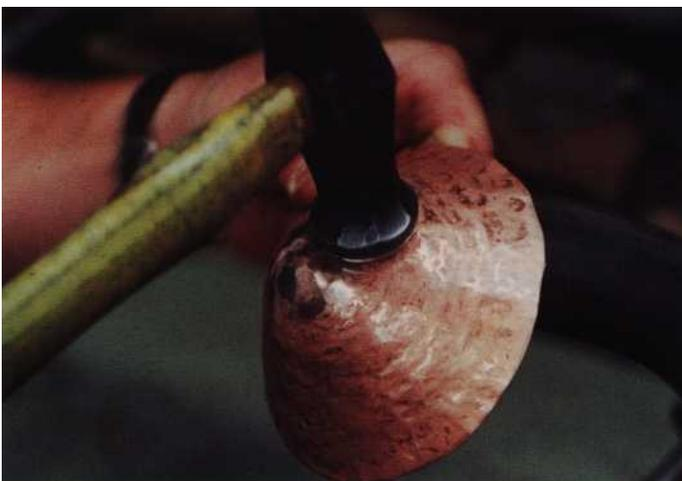
Figure 17. Planishing the shade cap. Notice the ugly working hammer marks left by the steel hammer in the "raising" process.
