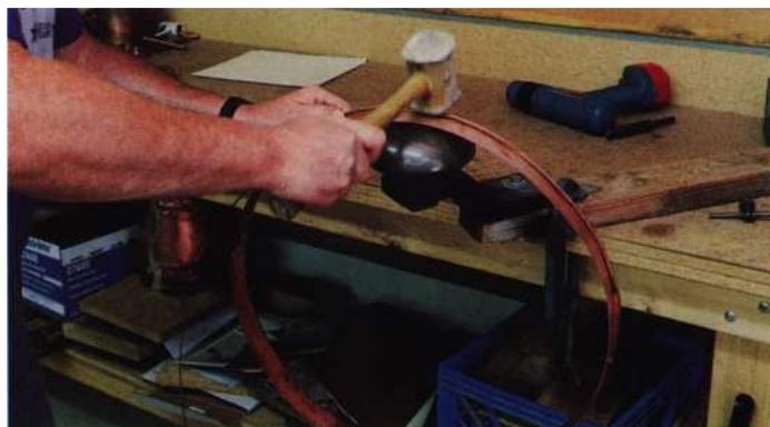
Figure 11. The rim of a later-period lamp starts out as a thin band that needs to have its top edge "raised" to the 45-degree conical shape. Here I am malleting over the edge to capture a wire.
