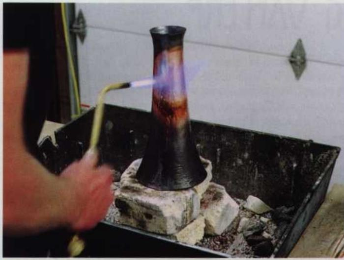
*Figure 5. The "trumpet" section of the "rivet-base" lamp being annealed in order to soften the copper so it can continue to be worked into the eventual shape.*
