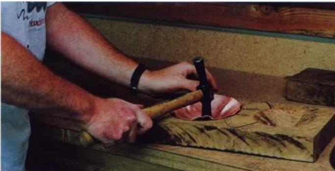
Figure 16. Sinking a copper disk into an oak form is the beginning phase in building the shade cap.
