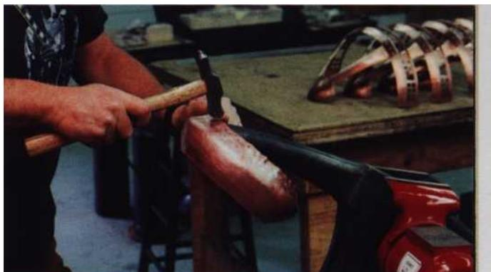
Figure 2. "Raising" the bottom bowl section of a "rivet-base" table lamp with a raising hammer onto the steel stake.
