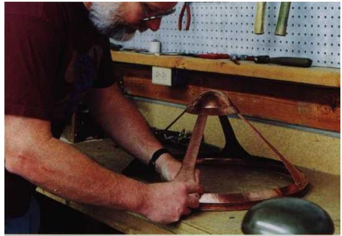
Figure 18. Fitting the battens to the completed shade with screws. These screws will be removed one at a time and replaced by copper rivets.
