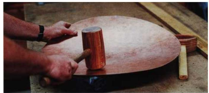
Figure 22. Regulating the inside surface of a van Erp "flat-top" shade. This is done with a wooden mallet over a sandbag.
